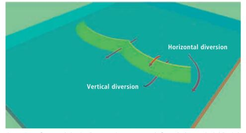
Figure 2. Current flows around a hanging silt screen: Main components are the flow under the screen (vertical diversion) and the flow around the screen's side edges (horizonal diversion).
