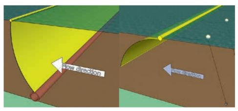
Figure 1. Standing (left) and hanging (right) silt screens.
