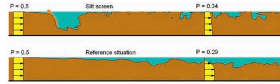
Figure 3. Example of application of percentage of reduction of *P* achieved by the screen. The yellow profiles represent values of *C*,, whereas the value of C, *z*, integrated over *z*, is given above each profile. In this situation,  $E_{in} = 32\%$  and  $E_{integrated} = -10\%$ .
