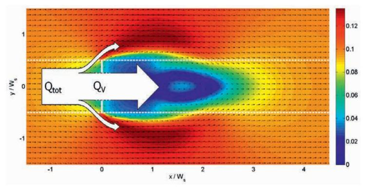
Figure 7. Example of a model current simulation with silt screen. The colours and vector arrows represent magnitude and direction of the depth-averaged flow velocity.
