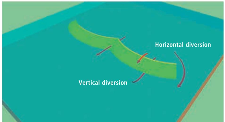
Figure 2. Current flows around a hanging silt screen: Main components are the flow under the screen (vertical diversion) and the flow around the screen's side edges (horizontal diversion).
