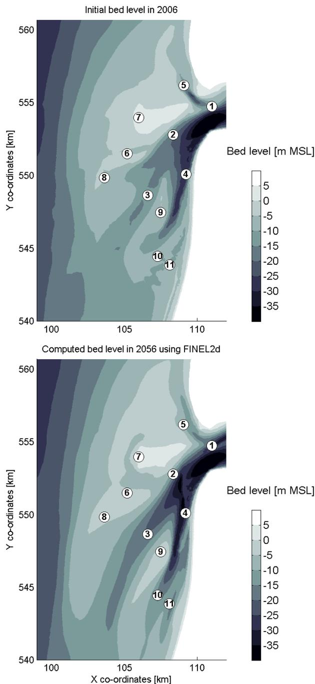
Figure 5. Initial bed level in 2006 and computed bed level in 2056 using FINEL2d
