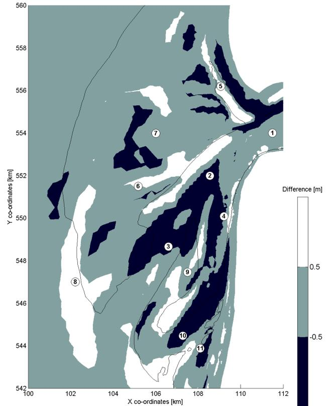
Figure 4. Computed erosion/sedimentation pattern
