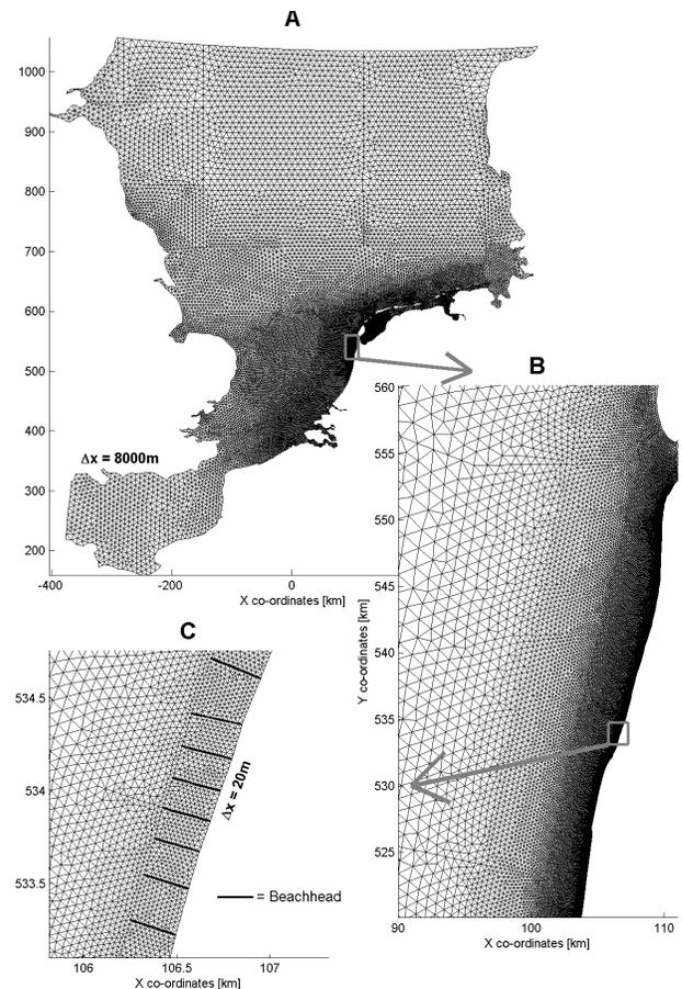
Figure 2. Grid schematisation from coarse (A) to fine (C)
