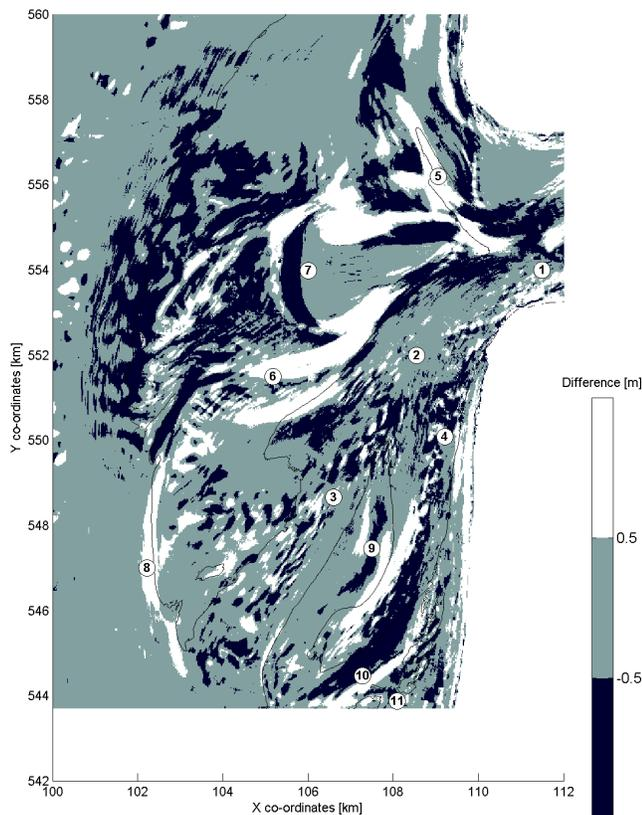
Figure 3. Observed erosion/sedimentation pattern 2000-2006
