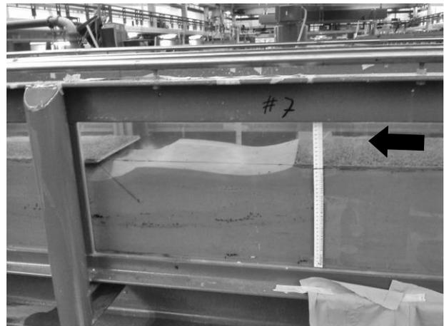
Figure 2: Flume experiment with scour hole. Flow is from right to left
