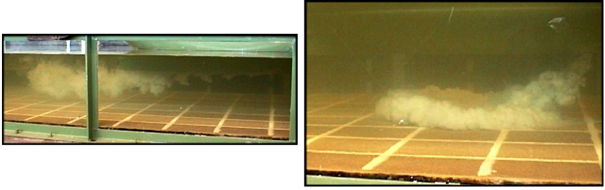
Figure 2.10: Characteristic pictures of both types of overflow plume spreading: mixing (left picture) and density-driven (right picture), Boot (2000).
