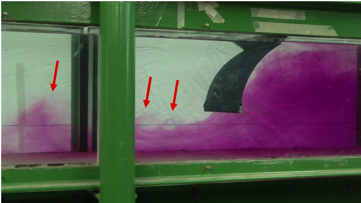
Figure 4.6: Snapshot of a dye injection during laboratory experiment 2B. Immediately downstream of the silt screen's bottom edge two curling vortices are visible, resulting from Kelvin-Helmholtz instability. Further to the left a more developed and diffused vortex can be seen.
