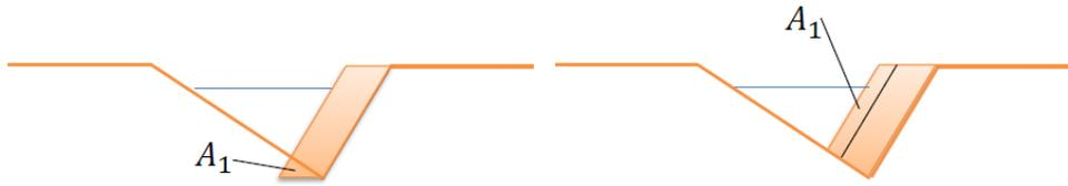
Figure 5.5: The correction of  $dy$  when the width of the bed becomes zero
