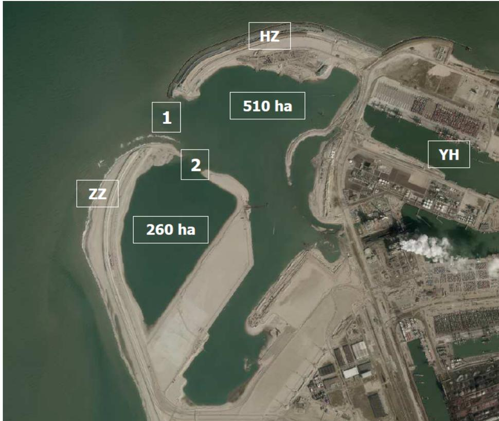
Figure 2.13: The 'Maasvlakte 2', with at number 1, the closure gap of the outer closure and number 2 is the closure gap of the 'compartimenteringsdam'
