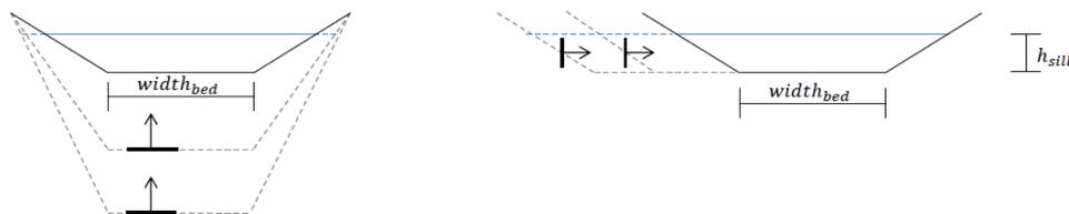
Figure 4.1: The left hand panel shows the vertical closure and the right hand panel shows the horizontal closure
