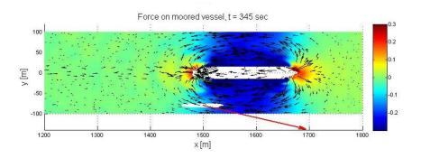
Example of computing the dynamic effect of a sailing vessel on a moored vessel, applying the Finite Element model FINEL2D.
