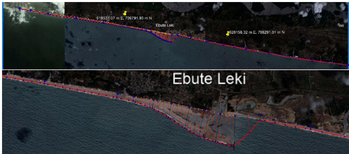
Figure 4.2: Coastline at the start situation as used in Unibest. Lower image is a detail of the breakwater of the upper figure.
