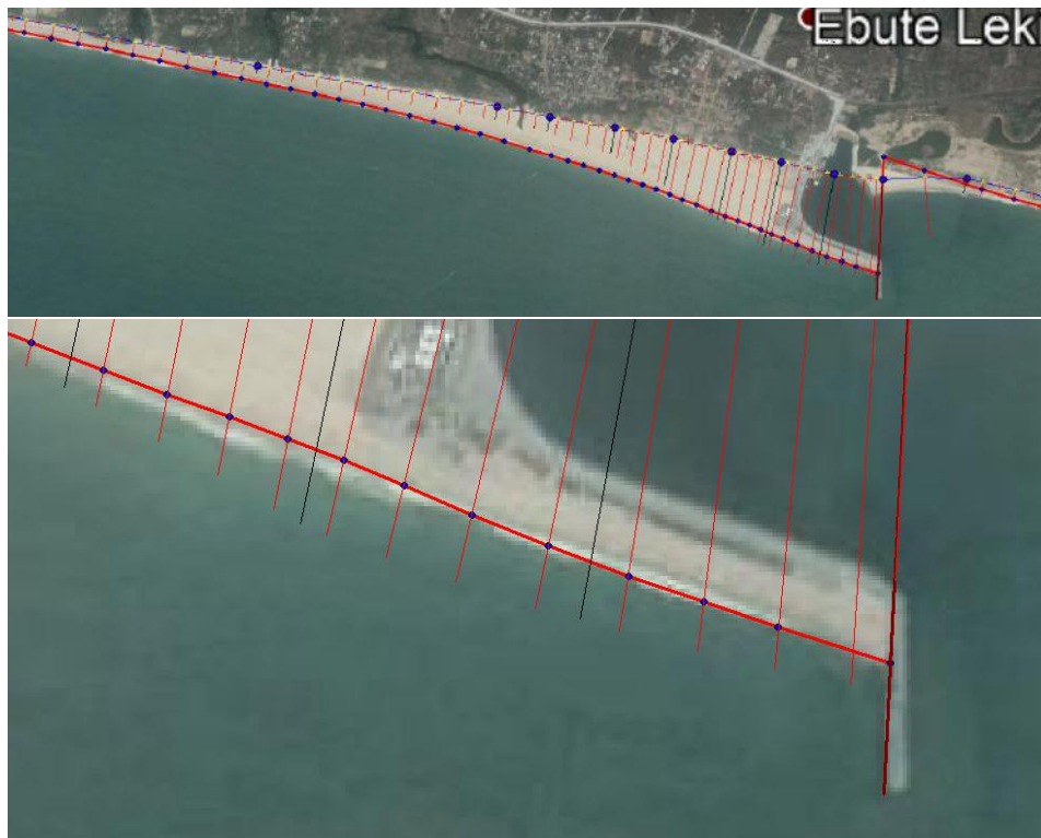
Figure 4.5: The situation after running Unibest for the period from March to December using the optimal settings. The upper figure shows the entire breakwater and the lower figure a detail of the sandbar only. The background shows the desired coastline used to validate the outcome.
