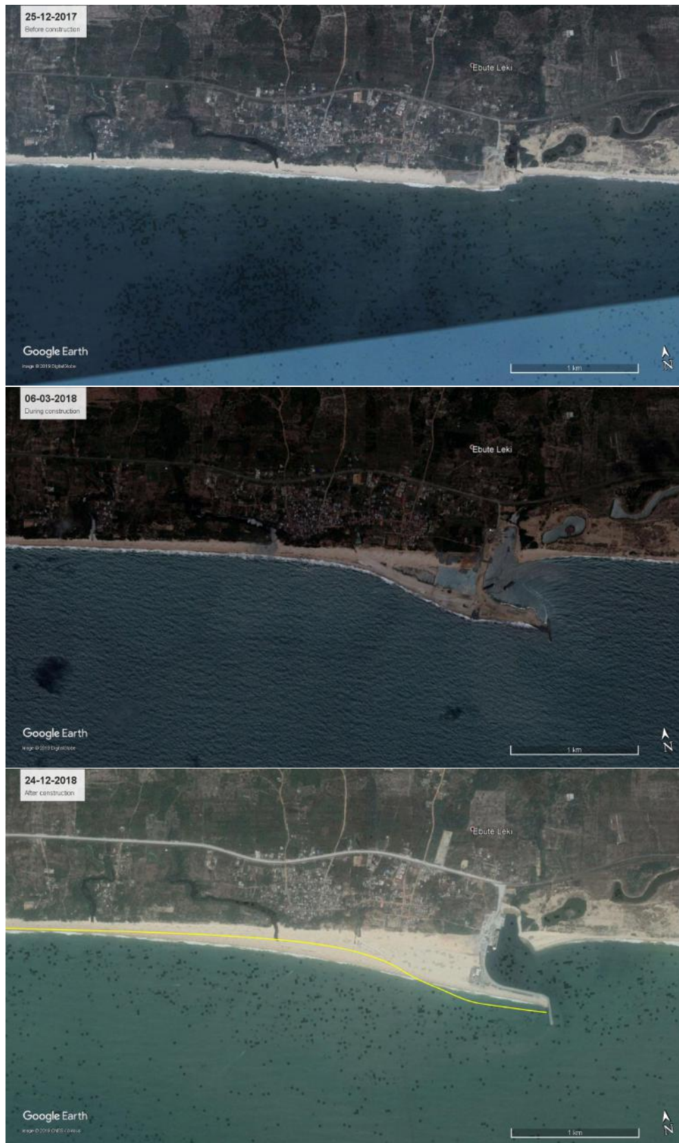
Figure 3.1: Three states of the construction and development after construction of the Lekki breakwater. The first image is taken before construction on 25-12-2017. The second image is taken during construction on 06-03-2018. The third image is taken some time after finishing the construction at 24-12-2018. The yellow line in the last image shows the coastline profile of 06-03-2018 (second image) (201, 2019)
