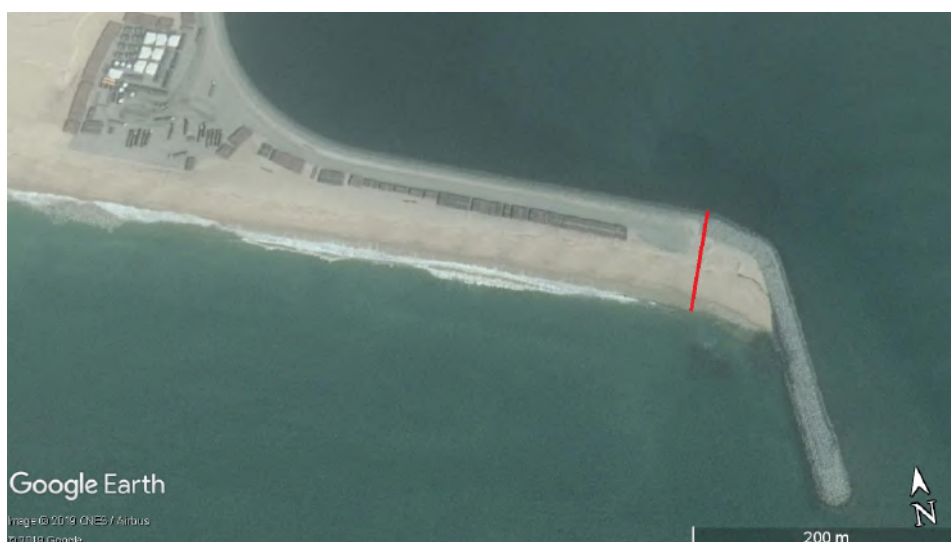
Figure 3.10: Detail of the sandbar at 24-12-2018. The red line indicates the narrowest part of the breakwater at around 90 meters from water to water.
