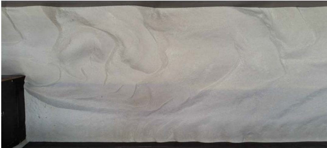
(a) Photograph of the final erosion and sedimentation pattern for experiment 6. The photograph is made at the just after the expansion, showing the bed until about one metre downstream of the expansion.
