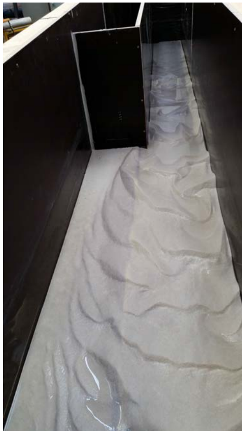
Figure 4.3: Photograph gives an overview of a typical final erosion and sedimentation pattern for an experiment with a moderate flow velocity, in this case for experiment 4.
