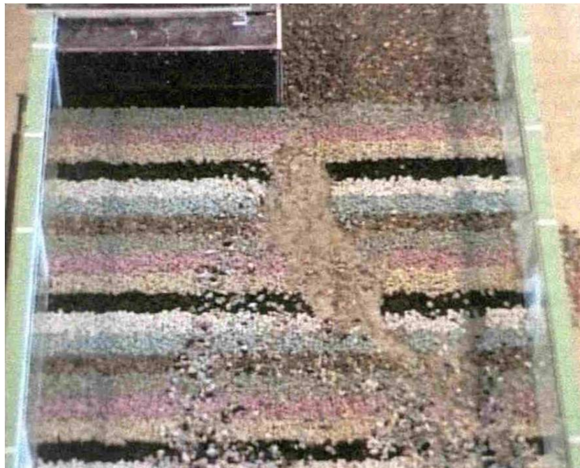
Figure 2.6: Damage pattern of gravel under a mixing layer caused by a lateral expansion. Figure from Zuurveld [23].
