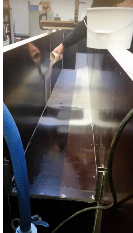
Figure 3.3: A photo of how epoxy was used to glue a layer of sediment to the bottom of the flume.
