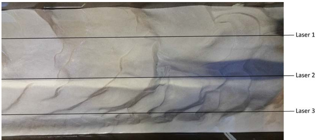
(b) Photograph of the final erosion and sedimentation pattern for experiment 7. The photograph is made at the end of the flume, showing the bed between 0.5 and 1.5 metres downstream of the expansion.
