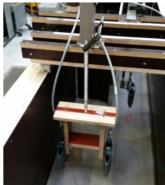
Figure 3.5: Photographs of the carriage placed on top of the flume. The left photo shows the positioning of laser 1 and the wheel that registers the location of the carriage. The right photo shows the positioning of laser 2 and 3.
