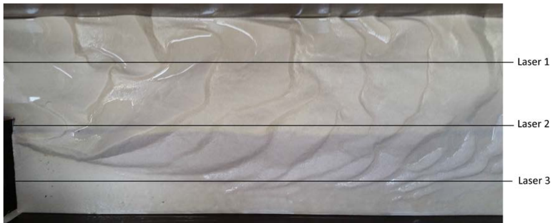
Figure 4.6: Photograph of the final erosion and sedimentation pattern for experiment 4, which was an experiment with a moderate flow velocity. The photograph shows the flume at the expansion and about the first 1.5 metres downstream of the expansion.
