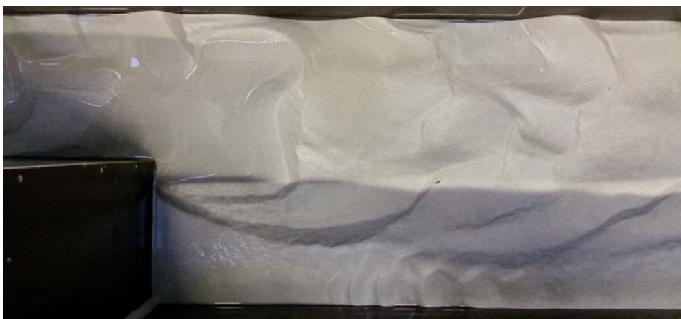
Figure 4.12: Photograph of the final erosion and sedimentation pattern for experiment 5, which was an experiment with a moderate flow velocity. The photograph shows the flume from just upstream of the expansion and the first metre downstream of the expansion.
