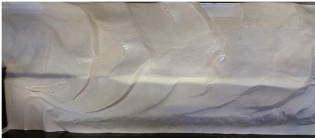
Figure 5.14: Photograph of the final erosion and sedimentation pattern for experiment 7. The photograph shows the flume at the expansion and the first metre downstream of the expansion.
