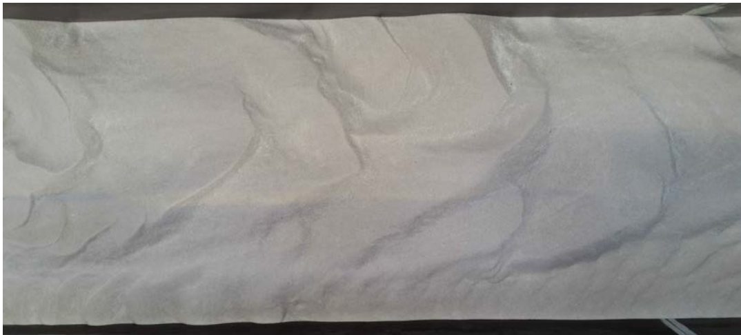
(b) Photograph of the final erosion and sedimentation pattern for experiment 6. The photograph is made at the end of the flume, showing the bed between 0.5 and 1.5 metres downstream of the expansion.
