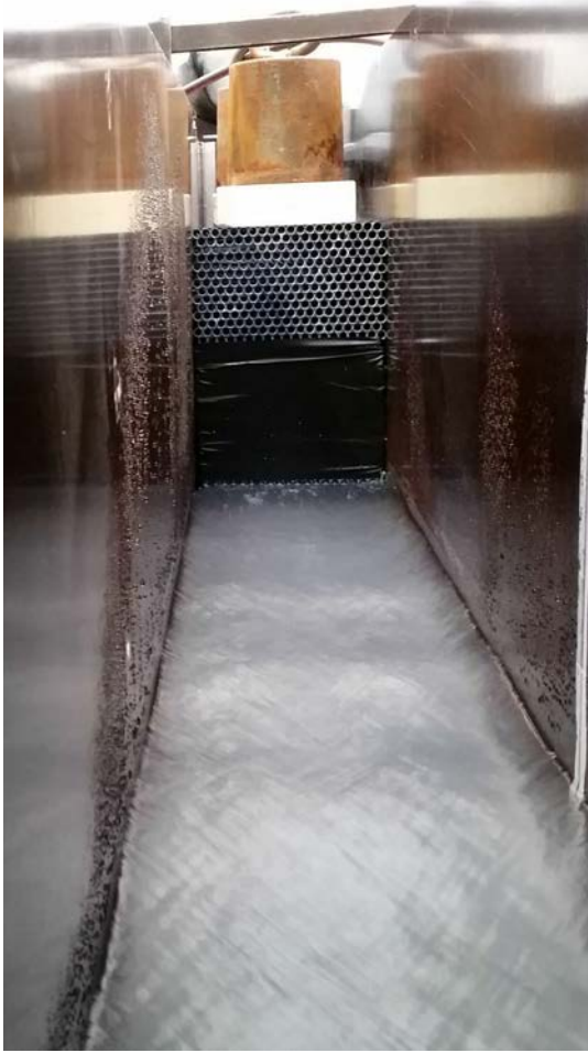
Figure 3.2: A photo of the flow straightener located at the beginning of the flume.
