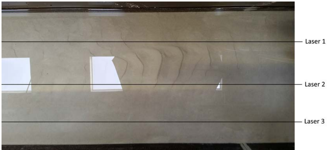
(b) Photograph of the final erosion and sedimentation pattern for experiment 2. The photograph is made at the end of the flume, showing the bed between 0.5 and 1.5 metres downstream of the expansion.
