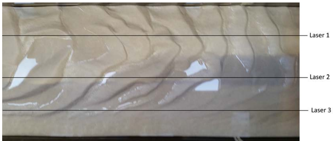
(b) Photograph of the final erosion and sedimentation pattern for experiment 4. The photograph is made at the end of the flume, showing the bed between 0.5 and 1.5 metres downstream of the expansion.
