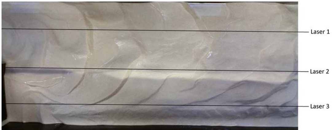
(a) Photograph of the final erosion and sedimentation pattern for experiment 7. The photograph is made at the just after the expansion, showing the bed until about one metre downstream of the expansion.
