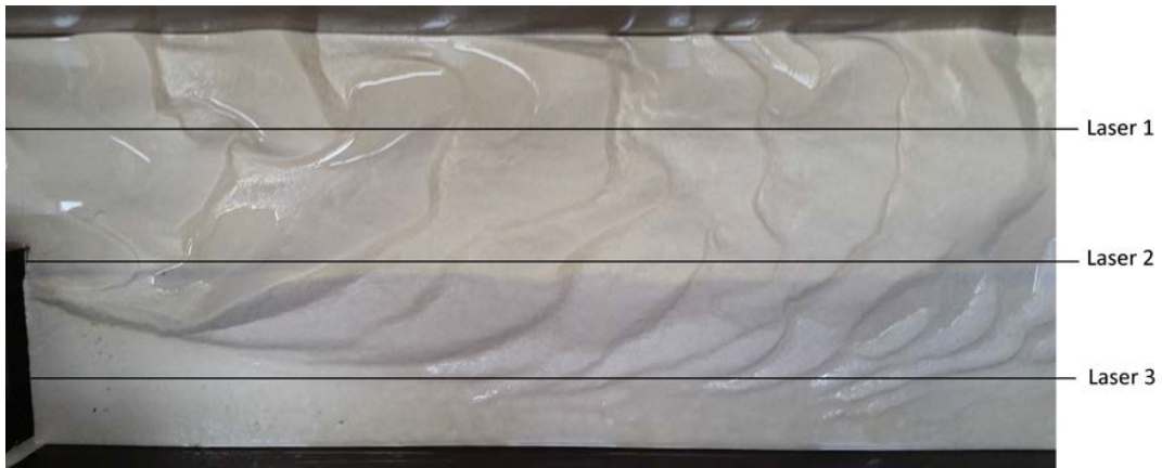
(a) Photograph of the final erosion and sedimentation pattern for experiment 4. The photograph is made at the just after the expansion, showing the bed until about 1.5 metre downstream of the expansion.
