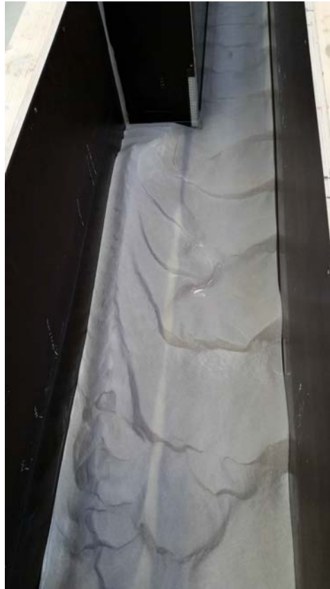
(a) Photograph of the final erosion and sedimentation pattern for experiment 8. The photograph is made at the end of the flume, facing in the direction of the expansion.
