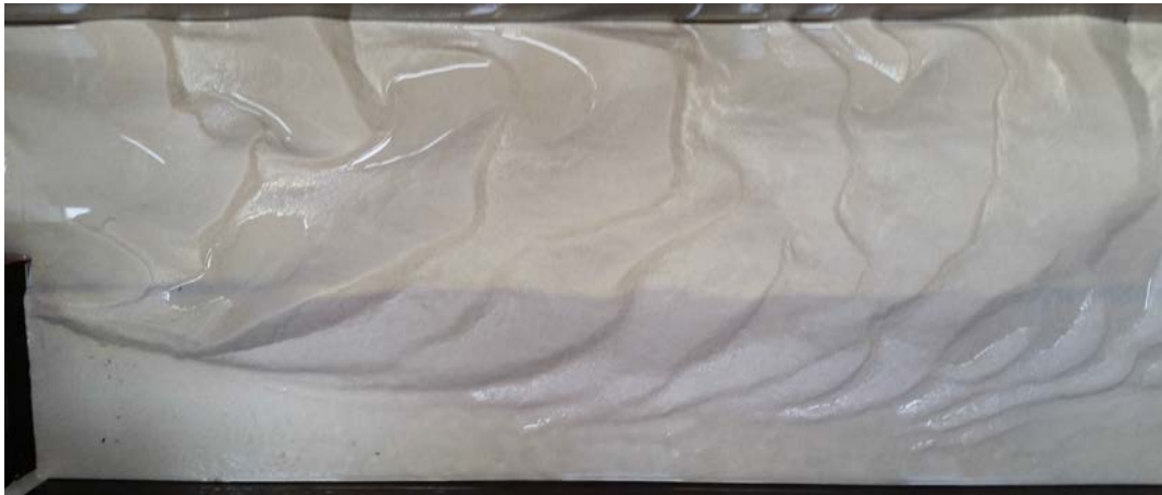
Figure 5.10: Photograph of the final erosion and sedimentation pattern for experiment 4. The photograph shows the flume at the expansion and about the first 1.5 metres downstream of the expansion. This is the same photograph as Figure 4.6.
