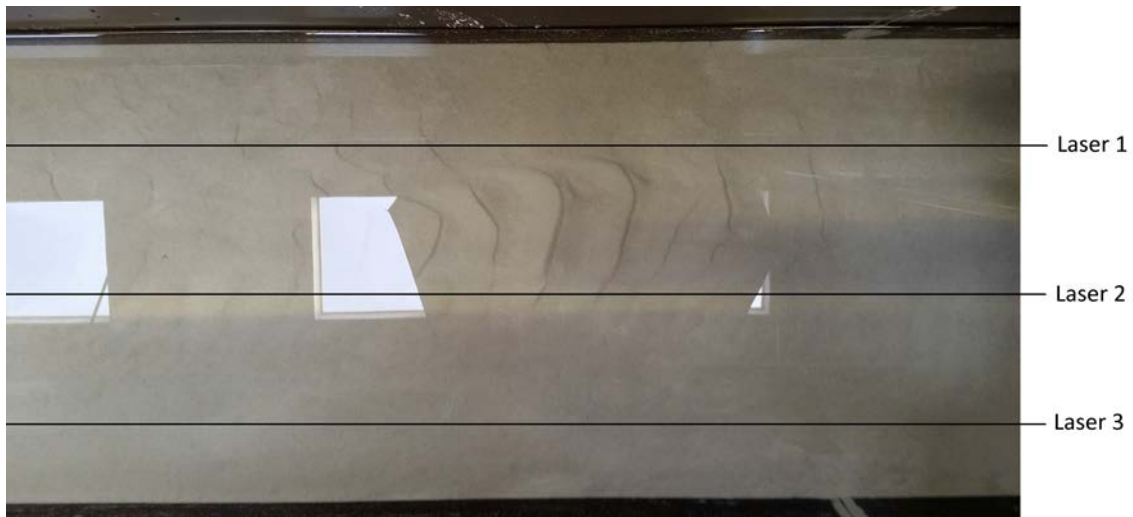
Figure 4.5: Photograph of the final erosion and sedimentation pattern for experiment 2, which was an experiment with a low flow velocity. The photograph is made at the end of the flume, showing the bed between 0.5 and 1.5 metres downstream of the expansion.
