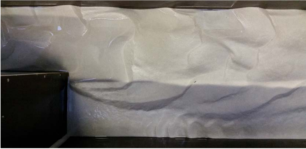
(a) Photograph of the final erosion and sedimentation pattern for experiment 5. The photograph is made at the just after the expansion, showing the bed until about one metre downstream of the expansion.
