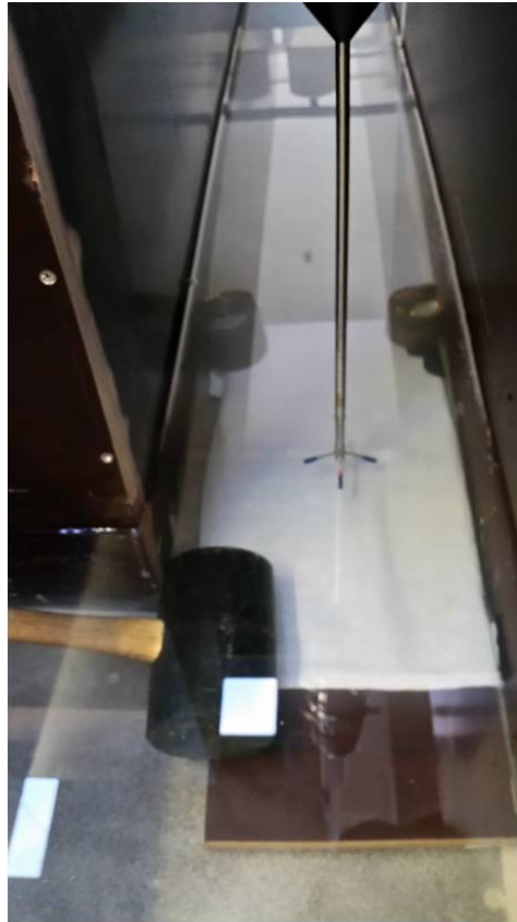
Figure A.6: Photograph of the set-up of the ADV and wooden board with cloth wrapped around it on the bottom of the flume.
