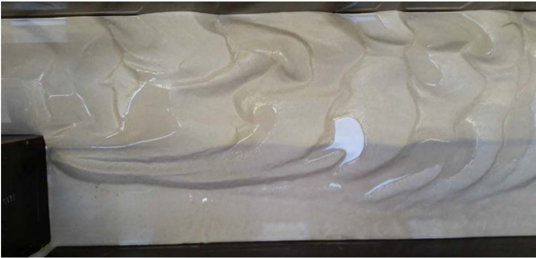
(a) Photograph of the final erosion and sedimentation pattern for experiment 4. The photograph is made at the just after the expansion, showing the bed until about one metre downstream of the expansion.
