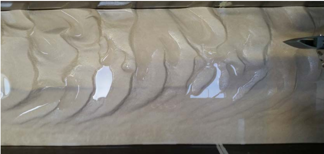
(b) Photograph of the final erosion and sedimentation pattern for experiment 4. The photograph is made at the end of the flume, showing the bed between 0.5 and 1.5 metres downstream of the expansion.
