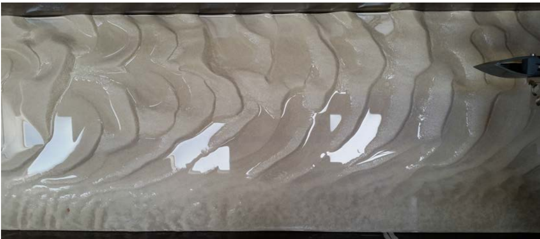
(b) Photograph of the final erosion and sedimentation pattern for experiment 3. The photograph is made at the end of the flume, showing the bed between 0.5 and 1.5 metres downstream of the expansion.
