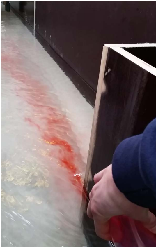
Figure 4.1: Determination of the flow pattern inside the mixing layer using dye.
