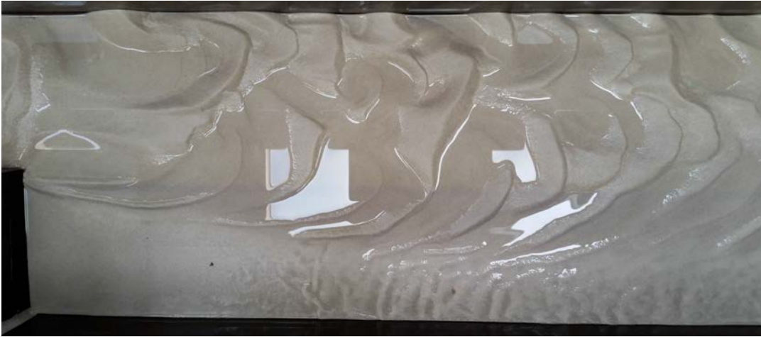
(a) Photograph of the final erosion and sedimentation pattern for experiment 3. The photograph is made at the just after the expansion, showing the bed until about one metre downstream of the expansion.
