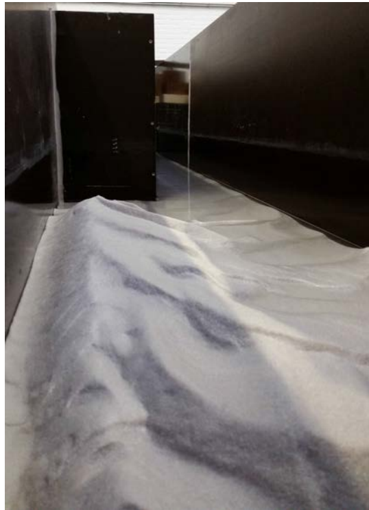
Figure 4.14: Photograph of the final erosion and sedimentation pattern for experiment 7, which was an experiment with a high flow velocity. The photograph is taken from the back of the flume, facing the expansion.
