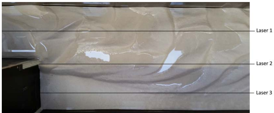
(a) Photograph of the final erosion and sedimentation pattern for experiment 4. The photograph is made at the just after the expansion, showing the bed until about one metre downstream of the expansion.
