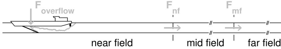
**Figure 2.1:** Schematic overview of the near field, mid field and far field of a dredging plume with the suspended sediment fluxes  $S_{j0}$ ,  $S_{nf}$ ,  $S_{mf}$  indicated.
